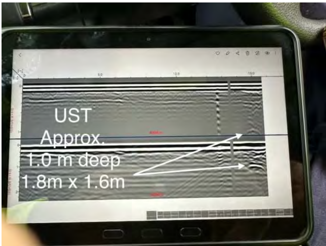
Photograph 8: Image of the GPR scan showing approximate depth of UST (image courtesy of A1 Locate Pty Ltd).
